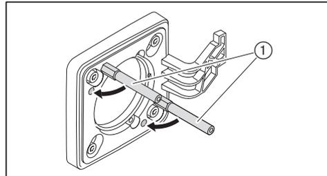
► Place burner into service position A [ch. 9.3].
